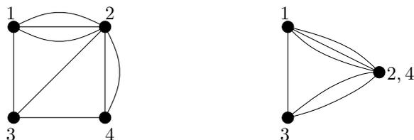
More precisely, the operation  $\text{Contract-Edge}(G, e)$  replaces a multigraph  $G$  by a multigraph  $G' = (V', E')$  with  $V' = V \setminus \{u, v\} \cup \{uv\}$  and  $E' := \{\{w, uv\} \mid w \in V \setminus \{u, v\}, \{w, v\} \in E\} \cup \{\{w, u\} \mid \{w, u\} \in E\} \cup \{\{w, x\} \mid \{w, x\} \in E, w, x \neq \{u, v\}\}$ .
